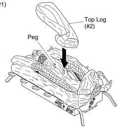
Figure 19 - Installing Top Log (#2)
